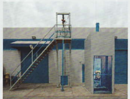
A drop test tower approximately 20' high was built to test body harnesses manufactured at Ultra-Safe, Inc.
