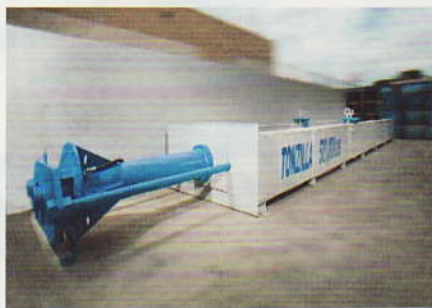
The business end of Marty Sharp’s homemade, 500,000 lb., pull tester.
