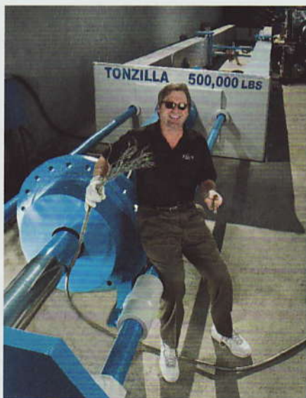
Marty Sharp and his pride and joy, Tonzilla, a 500,000 lb. pull tester he constructed himself using mostly surplus parts and scrap metal.
